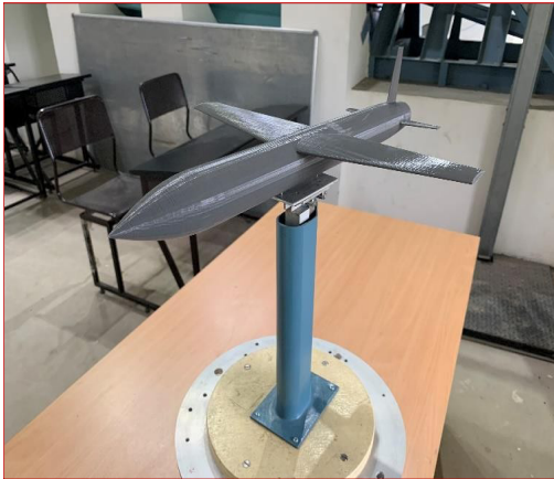
Figure 10. Image of the 3D printed model placed in 6 component balance
