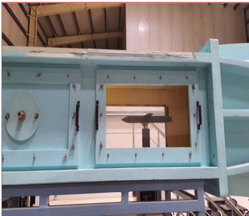
Figure 12. 3D printed model in the test section
